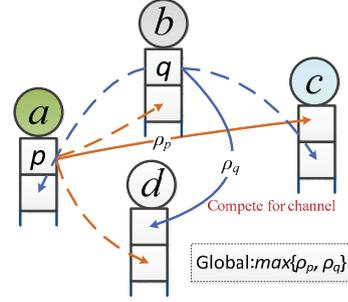
Figure 3: An illustrating example with four nodes for explaining the global algorithm. The links formed among node  $a, b, c$  should compete for the media.
