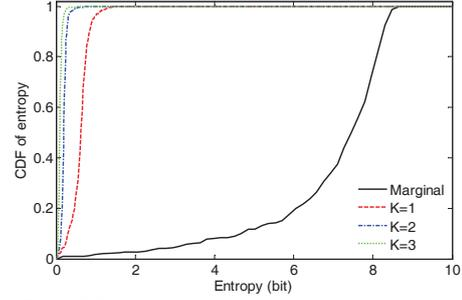
Figure 1: The CDFs of marginal entropy and conditional entropies of a vehicle positional state. The grid size is 200 m×200 m, and the number of vehicles is 500.
