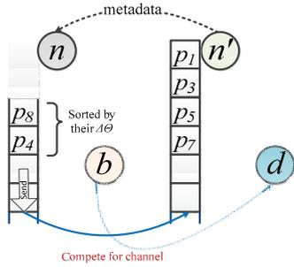
Figure 4: An illustrating example for explaining the distributed algorithm at node  $n$ . The link between  $n$  and  $n'$  may compete for the media with the link between  $b$  and  $d$ .
