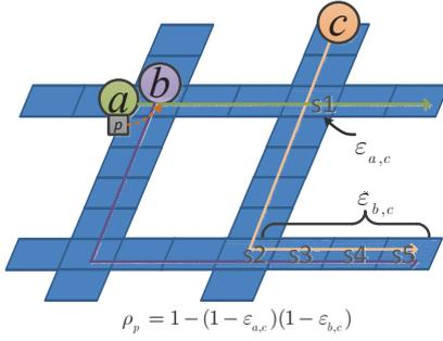
Figure 2: An illustrating example of calculation for encounter probability and delivery probability.
