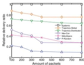
Figure 10: Delivery ratio vs. amount of packets, with Shanghai bus dataset.
